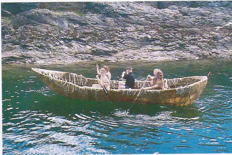
The Flyer a hide 'Neolithic' Currach built by Peter Faulkener
